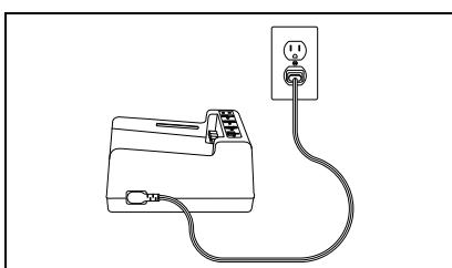
Only use the cord set that was supplied with the charger. At first use, verify that the plug type matches the receptacle.
